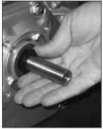
Install the pump slinger (12706) on to the drive unit shaft. The slinger should be slid all the way back on the shaft of the drive unit so that the slinger covers the step on the drive unit shaft as shown.
