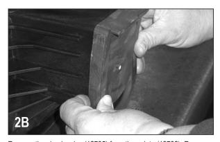
Remove the check valve (12705) from the volute (13702). Remove the one upper volute screw (12900) and the two smaller volute screws (12725) from the volute. Remove the volute from the remaining pump assembly.
