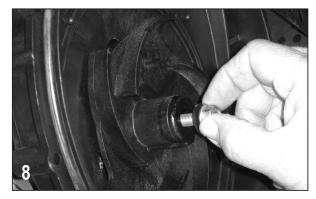
Secure the impeller to the drive unit shaft with the impeller bolt gasket (12774VA) and impeller bolt (12765A). Tighten the impeller bolt until snug (31-55 in lbs).
