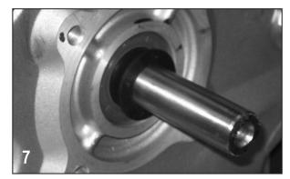
At this time, it may be necessary to polish the drive unit shaft to remove any corrosion that may have formed.
