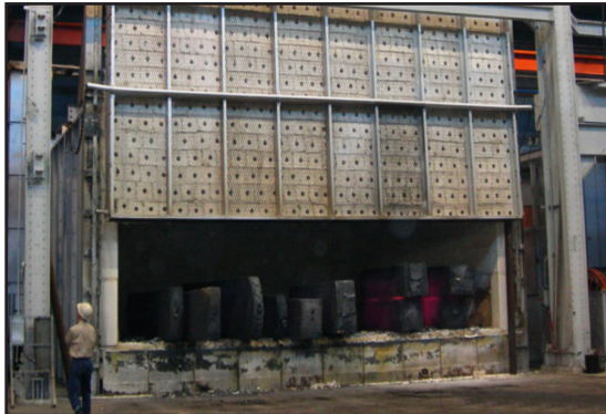
Heat treating alloys requires a controlled rate of heat-up and cool down.
