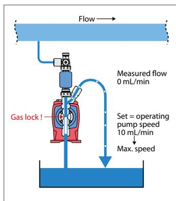
When a large volume of gas enters into the pump chamber, pump output will go to "zero" until the gas bleeds out. The feedback control increases pump speed, reducing the bleed time and quickly re-priming the pump.
