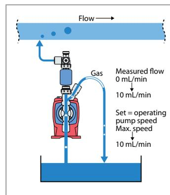
After the gas has been purged, the EFS sensor will begin to measure flow. Feedback from the sensor controls the pump, slowing it back down so the flow rate meets the set value.
