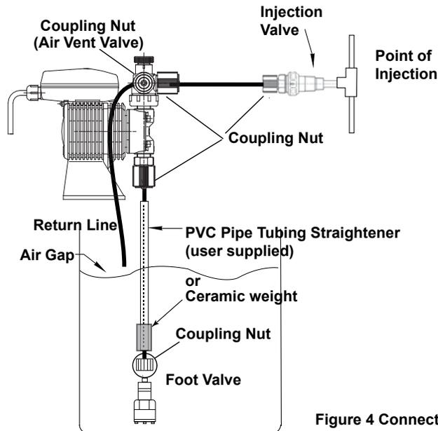
Figure 4 Connection Tubing
