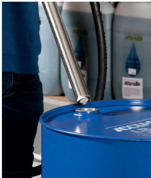
The closing of the backflow valve prevents the lubricant from flowing back out of the pump into the drum.
