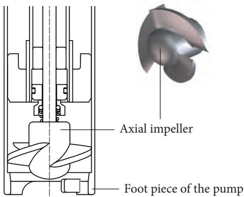
F/FP 430 with mechanical seal and axial impeller
