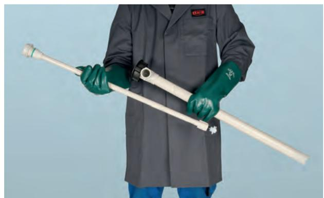
With just three hand movements the pump can be disassembled into inner tube (complete) and outer tube.
