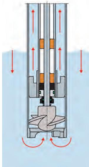
The mechanical seal prevents medium from getting into the inner tube while pumping.
