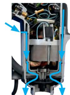
The arrows show how the cooling air flows through the interior of the motor and the chambers of the double housing.
