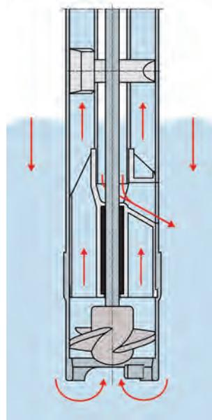
Optimal flow of the medium in the inner tube due to relief openings in the bearing housing.
