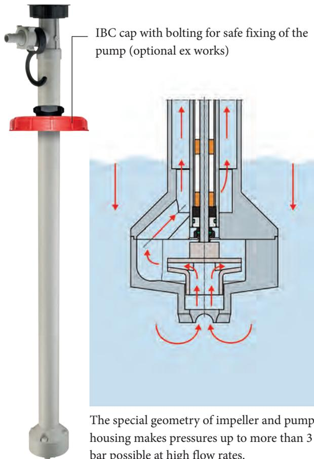
The special geometry of impeller and pump housing makes pressures up to more than 3 bar possible at high flow rates.
