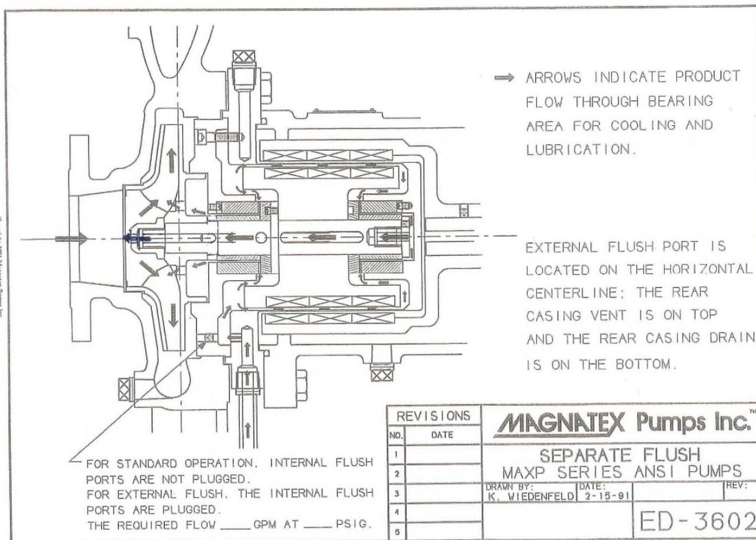
Connect the separate flush piping to the 1/2" NPT flush connection located 90° to the right on the rear casing flange, as viewed from the pump suction end.
