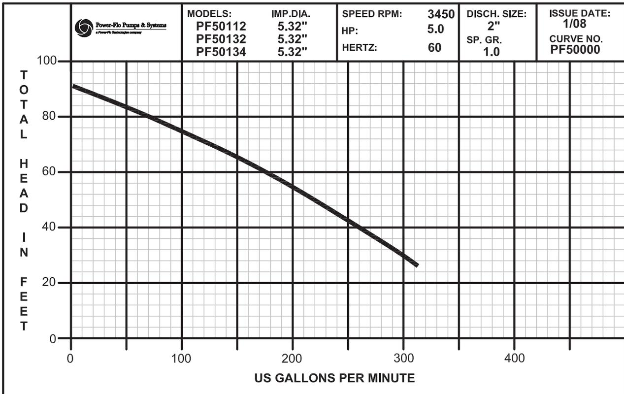
**Dewatering Pumps - 5HP - 3450RPM - 60Hz**
