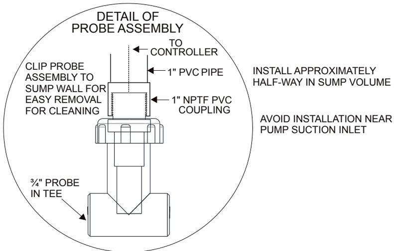
Figure 5 Typical Cooling Tower Installation Submersion Sensor
