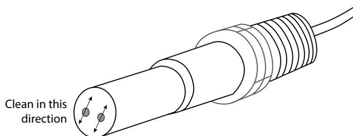
**Figure 14** Cleaning a flat contacting conductivity electrode
