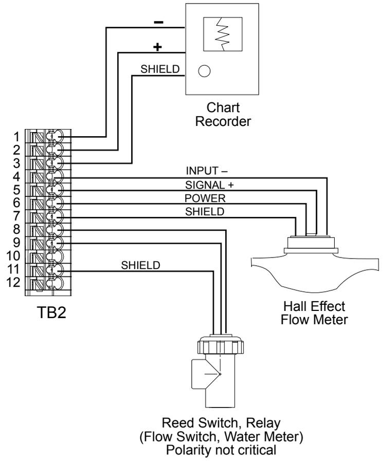
Figure 10 Digital Input and Analog Output Wiring
