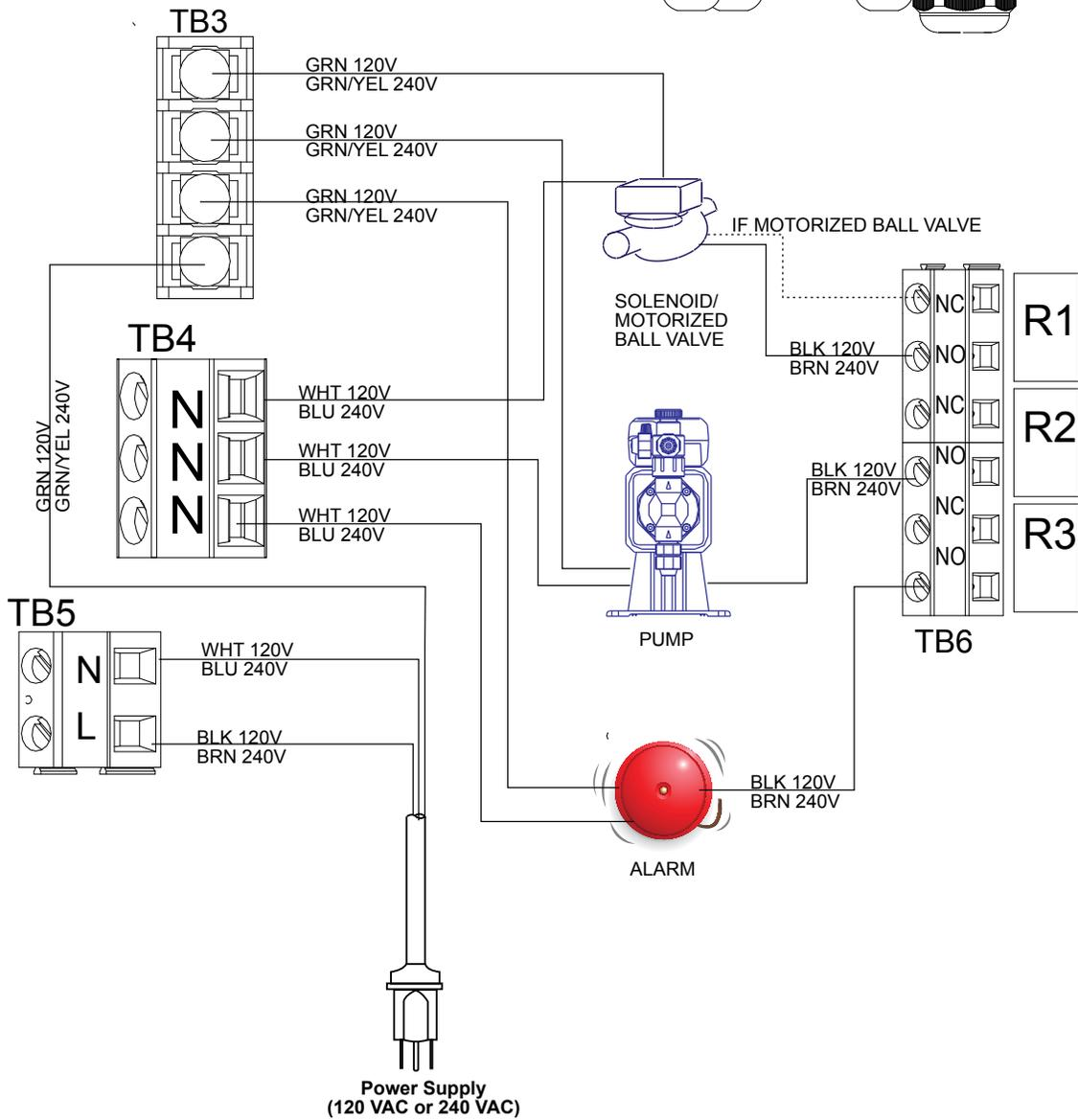
Figure 11 W100 AC Power & Relay Output Wiring
