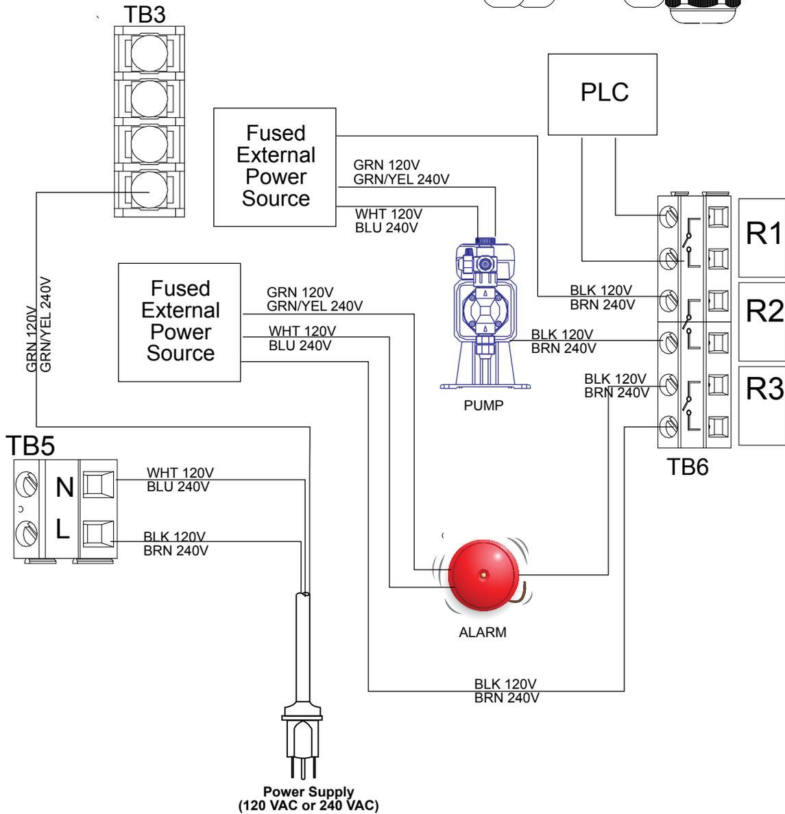
**Figure 12 W110 AC Power & Relay Output Wiring**
