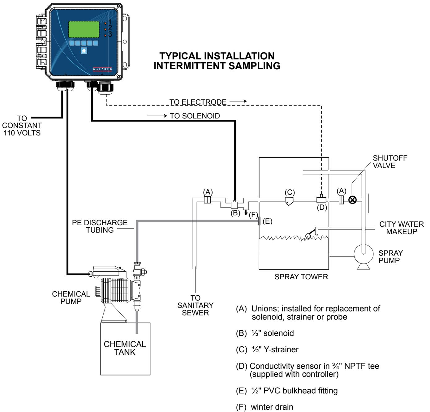
**Figure 6 Typical Cooling Tower Installation Intermittent Sampling**
