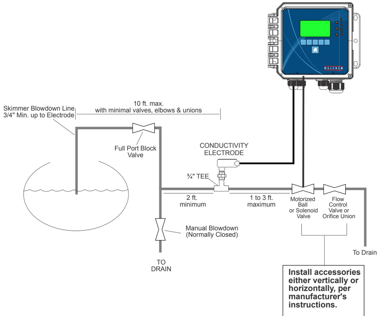
**Figure 3 Typical Boiler Installation Intermittent Sampling**
