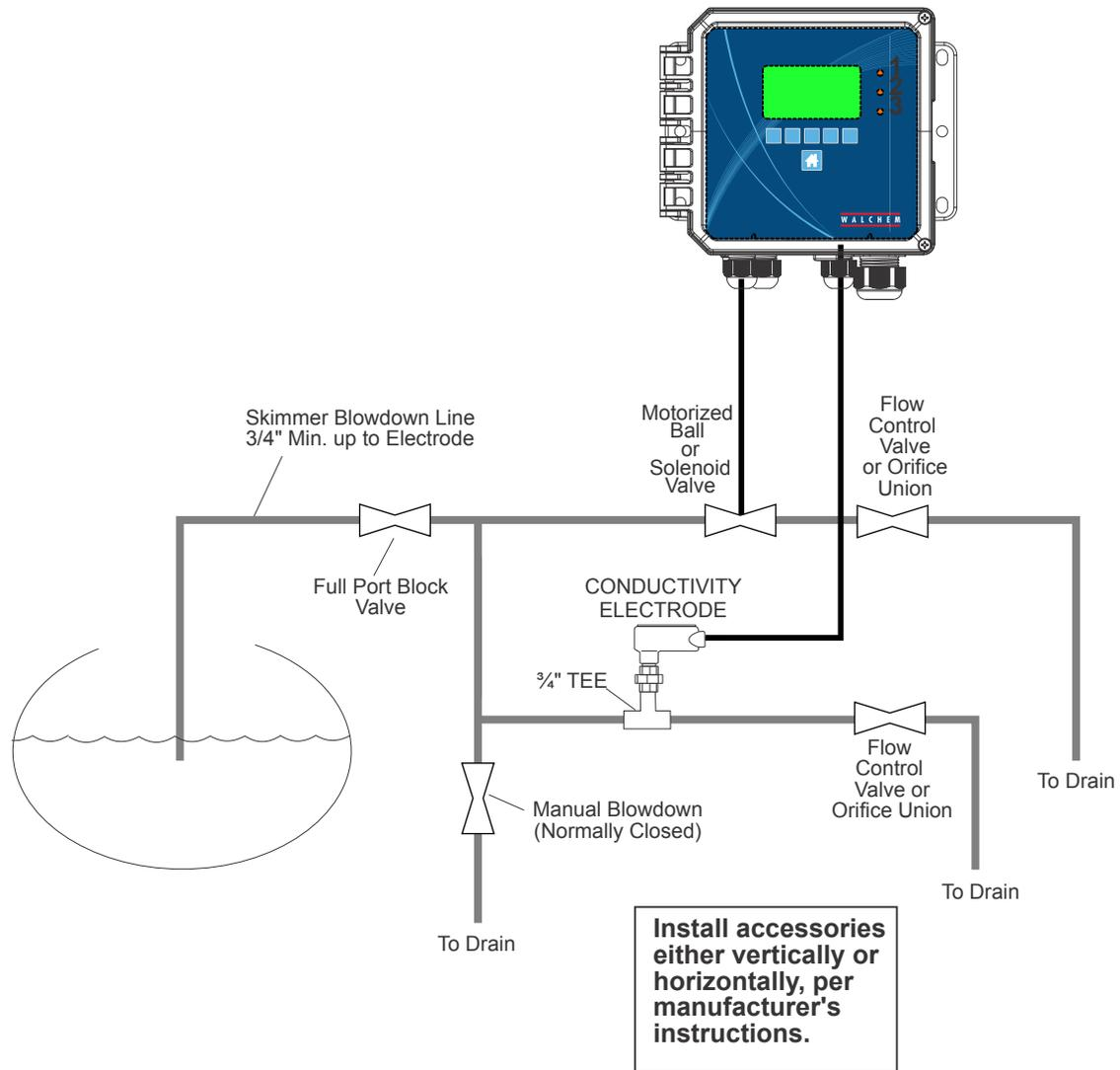
**Figure 4 Typical Boiler Installation Continuous Sampling**
