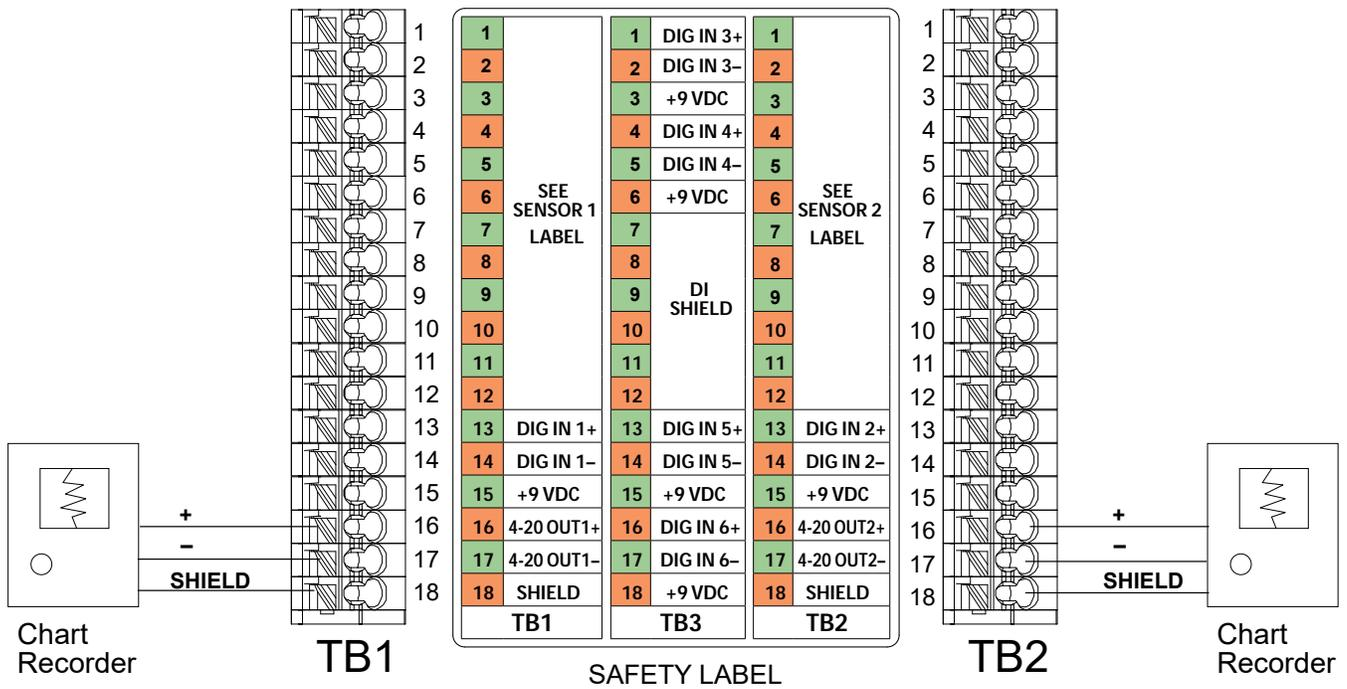
Figure 18 Analog Output Wiring
