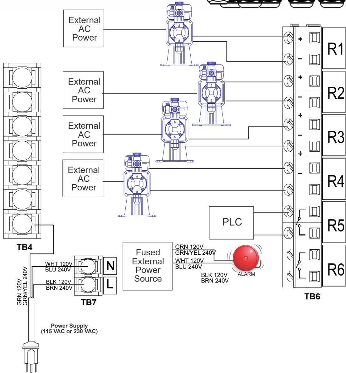
Figure 17 W640 AC Power & Relay Output Wiring
