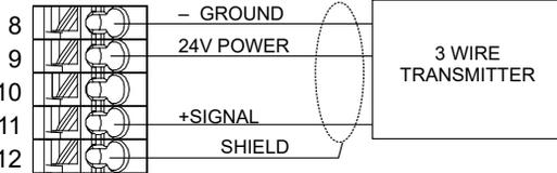
**NOTE:** To program the combination card analog input, you must go to Inputs menu, then enter the analog input (S13 or S23), scroll down to Transmitter, and select the type of transmitter from the list.
