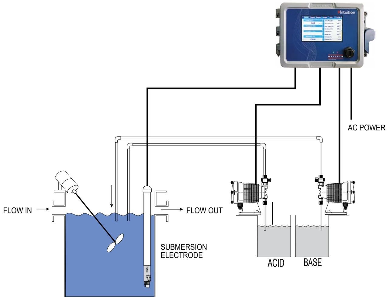
**Figure 2 Typical Installation – Cooling Tower Submersion**
