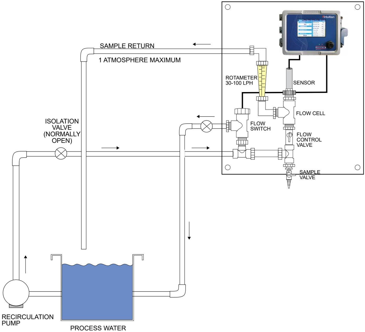
**Figure 3 Typical Installation – Disinfection Sensor**
