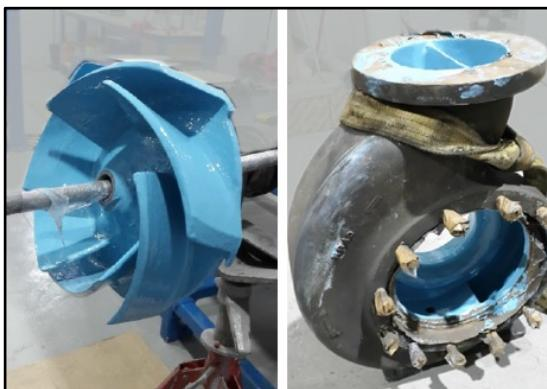
*In process: manual apply three coats of ARC HT-S.*
