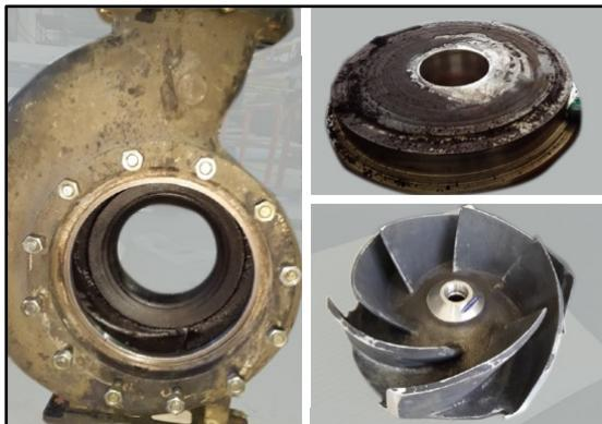
*Before: Pump and back plate showing scaling, impeller is new.*
