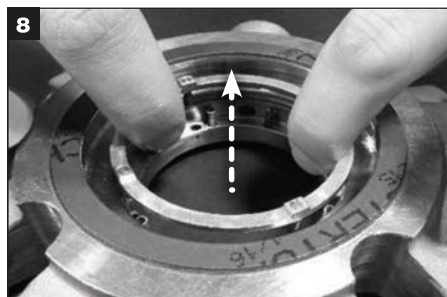
Remove the follower assembly from the gland and set it aside.
