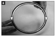
For seals with Bushing kit: Apply a thin film of white grease to the bushing O-Ring (Y) and install into the groove on the bronze bushing. IMPORTANT: Ensure the O-Ring is completely seated and fully captured within the O-Ring groove. The O-Ring may appear to be oversize when installing and will need to be worked in.
