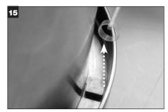
Remove drive from drive lugs in the sleeve and discard.
