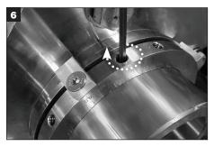
Tighten three dog point set screws ① (see inset image, marked with a dimple) evenly with the hex key provided.
