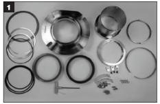
Tools required for assembly of seal: Hex key and two types of grease (supplied with seal); lint-free cloth, tweezers or a thin pick (supplied by customer; for installation of O-Rings and drive tube). Clean all metal components with an approved solvent, including all gasket and O-Ring surfaces. Place metal components and all spare seal components on a clean dry surface.
