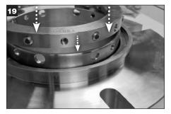
Place the lock ring on top of the sleeve and align the three vertical dimples on the outer diameter of the lock ring with the notch on the top edge of the sleeve.
