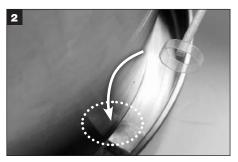
Pick up the drive tube (use tweezers if necessary) and install onto each of the lugs in the sleeve assembly. Ensure the drive tube are fully seated on the lugs.
