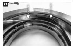
Align the pins on the follower plate with the marked, **635 SXC grease** filled holes in the gland and press down the plate into the gland until the follower plate rests on the springs.
