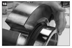
Lift up on the gland and hold the bottom of the sleeve to invert and gently set down to initiate contact between the stationary and rotary faces.
