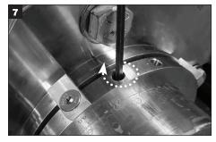
Tighten cup point set screws (2) evenly with the hex key provided. **IMPORTANT: After all sets screws have been tightened by hand, retighten with a torque wrench: to 13,6 – 15,3 Nm (120 – 135 in-lbs.)**
