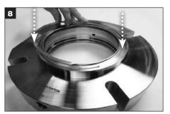
For seals with Bushing kit: Install the snap ring on top of the bushing and into the groove in the gland to secure the bushing into the gland.
