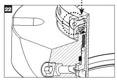
Press down on the top of the gland to compress the assembly and turn each centering clip to engage the groove on the top of the gland and hand-tight the centering clip flat head screw. Repeat this step for all centering clips. Retighten with a torque wrench: **8 Nm (71 inch-pounds)**.
