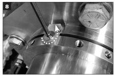
Remove all flat head screws and centering clips and retain for future use when making impeller adjustments and/or seal removal.
