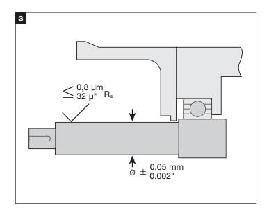
Remove all sharp corners, burrs, and scratches on the shaft, especially in areas where the O-Ring will slide, and polish if necessary to achieve a 1,1 micron (45 microinch) Ra finish. Make sure the shaft or sleeve diameter is within 0,05 mm (.002") of nominal.
