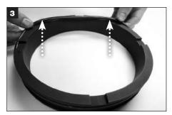
Apply a thin film of **white** grease to the rotary O-Ring (W) and install into the groove on the outer diameter of the rotary face. Ensure cushions are on the back of the rotary face.
