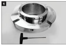
Tools required for disassembly of seal: Hex key (supplied with seal); tweezers and a curved pick (supplied by customer; for removal of O-Rings and drive tube).
