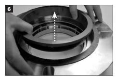
Remove the stationary seal ring from the gland and discard.
