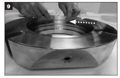
For seals with Injector option: Invert the gland. Compress and overlap the ends of the injector, position the splits opposite the F (flush) port and install in the gland groove. **IMPORTANT: The** injector should snap into place. Ensure the split ends do not overlap when fully installed.
