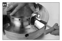
Install the centering clips on the outer diameter of the lock ring with the centering clip flat head screws.
