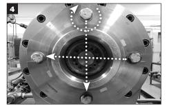
Tighten the gland bolts evenly. **IMPORTANT:** The gland bolts must be tightened before tightening the set screws onto the shaft. **Gland bolt torque is dependent on application. IMPORTANT:** Piping connections should not be made prior to tightening the gland bolts.
