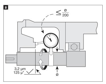
If possible, attach a base dial indicator to the shaft and rotate both the indicator and shaft slowly while reading the runout of the stuffing box face. Misalignment of the stuffing box face relative to the shaft should not exceed 0,005 mm TIR per mm (.005 in per inch) of shaft diameter.
