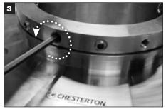
Remove all cup point and dog point set screws from the lock ring and discard.
