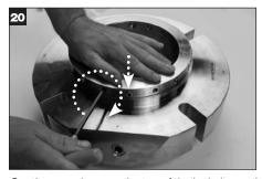
Gently press down on the top of the lock ring and tighten the dog point set screws and then the cup point screws with the hex key supplied with the seal. **IMPORTANT:** The set screws should be tightened just enough to ensure that they are secure but should not protrude into the inner diameter of the sleeve.
