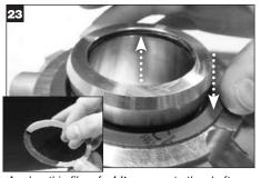
Apply a thin film of **white** grease to the shaft O-Ring (V) and install on the sleeve inside diameter O-Ring groove. Peel off the adhesive backing from the gland gasket and install in the gland gasket recess.
