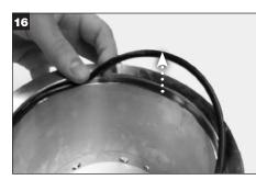
Remove the shaft O-Ring (V) from the sleeve and discard.
