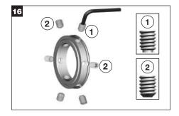
Install the dog point set screws ① into the screw holes marked with a dimple on the outside diameter of the lock ring. Install the cup point set screws ② into the remaining holes in the lock ring. **IMPORTANT: The screws should not protrude into the inner diameter of the lock ring prior to installing onto the seal sleeve.**
