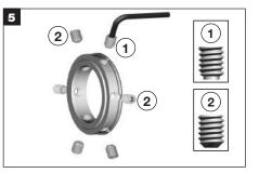
IMPORTANT: dog point set screws ① must be tightened FIRST and cup point set screws ② must be tightened last. Dog point set screw locations are marked with a dimple on the outside diameter of the lock ring, next to the screw holes.
