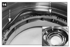
Apply a thin film of **white** grease to the stationary face O-Ring (X) and install into the groove in the gland above the follower plate assembly.
