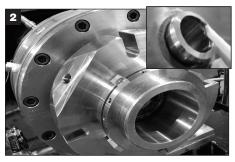
Apply a thin film of **white** grease to the shaft O-Ring (V) and slide seal onto the shaft by pushing on the gland. **CAUTION: Ensure that all set screws are engaged through the sleeve but do not protrude into the sleeve inside diameter bore.**
