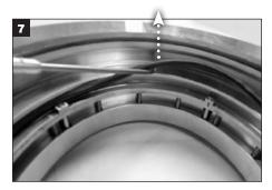
Remove the O-Ring (X) from the gland O-Ring groove and discard.
