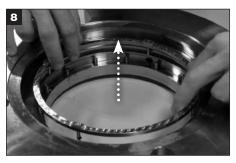
Remove the follower assembly from the gland. Remove and discard drive tubes from drive lugs, set follower assembly aside.
