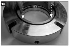
Align the slots on the stationary face with the lugs on the follower plate and gently compress the stationary face down until it is fully seated. **CAUTION: Improper alignment will result in chipping at the slot edges of the face.** Clean the stationary face with a lint-free cloth and an approved cleaning solvent that complies with local and site regulations. **CAUTION: Do not compress drive tube.**
