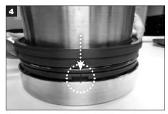
Align the mark on the rotary face with the notch on the sleeve. Slide the rotary face down to the sleeve and gently compress until it is seated. The sleeve drive lugs should engage the slots on the rotary face. **CAUTION: Do not compress drive tube.**
