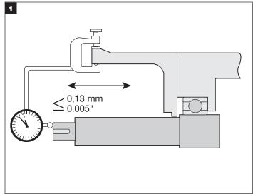
If practical, place the dial indicator tip on the end of the shaft sleeve or on a step in the shaft to measure end play. Alternately push and pull the shaft in the axial direction. If the bearings are in good condition, end play should not exceed 0,13 mm (.005").
