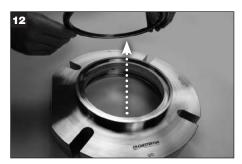
For seals with Bushing kit: Remove the bushing and bushing O-Ring (Y) from the gland bore and discard.
