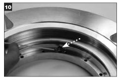
Fill the four evenly spaced holes, marked by dimples, with the 635 SXC grease supplied with the seal. Wipe off excess grease. Helpful Hint: Use the follower plate as a guide to confirm that grease will be applied to the correct holes.
