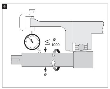
Use a dial indicator to measure the shaft runout in the area where the seal will be installed. Runout should not exceed 0,001 mm TIR per mm (.001 in per inch) of shaft diameter.
