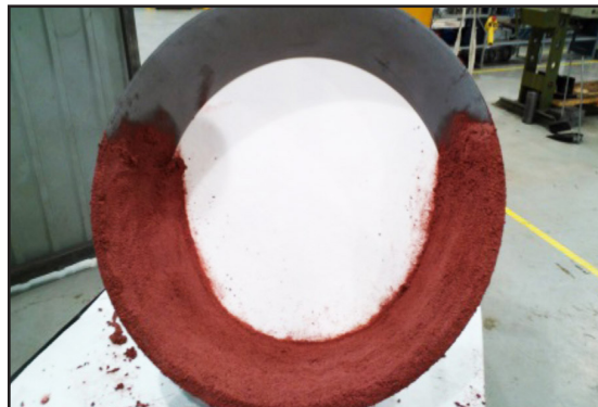
Side plate during ARC T7 AR application.
