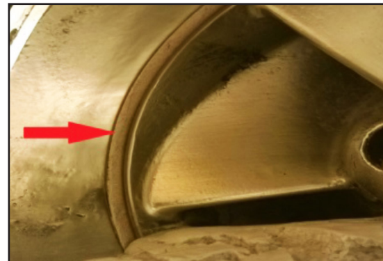
No loss of tolerance between impeller and side plate protected with ARC T7 AR.
