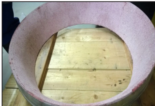
Side plate after machining the ARC T7 AR.
