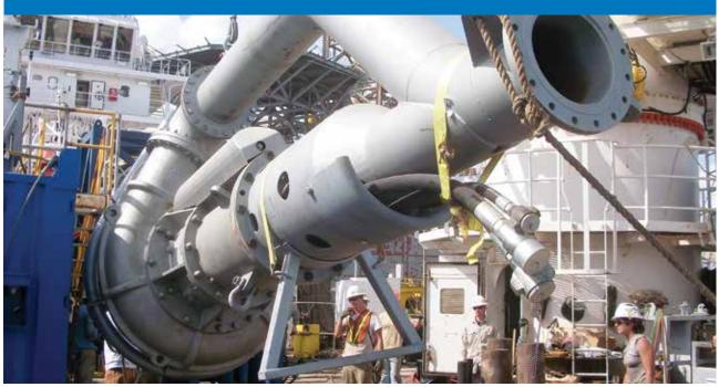
The **Toyo submersible DP series** and its hydraulically driven cousin the **TO series** were specifically designed to pick up and transport abrasive materials with the least amount of water.
