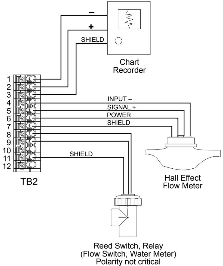
Figure 12 Digital Input /Analog Output Wiring
