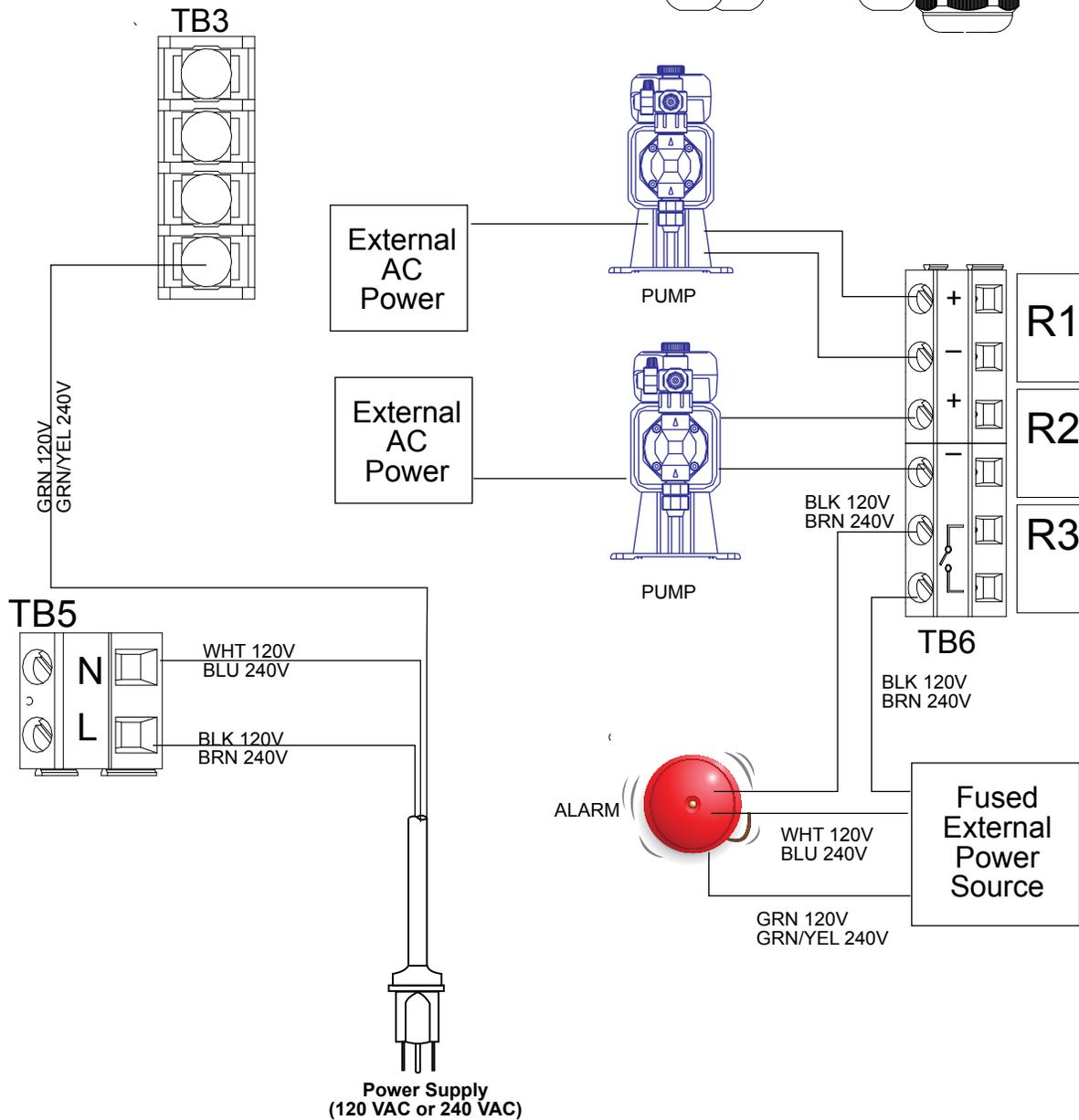
**Figure 15 W120 AC Power & Relay Output Wiring**
