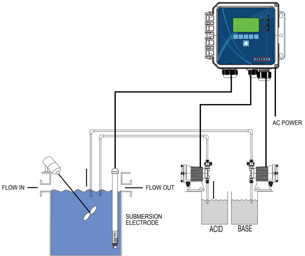
**Figure 3 Typical Submersion Sensor Installation**
