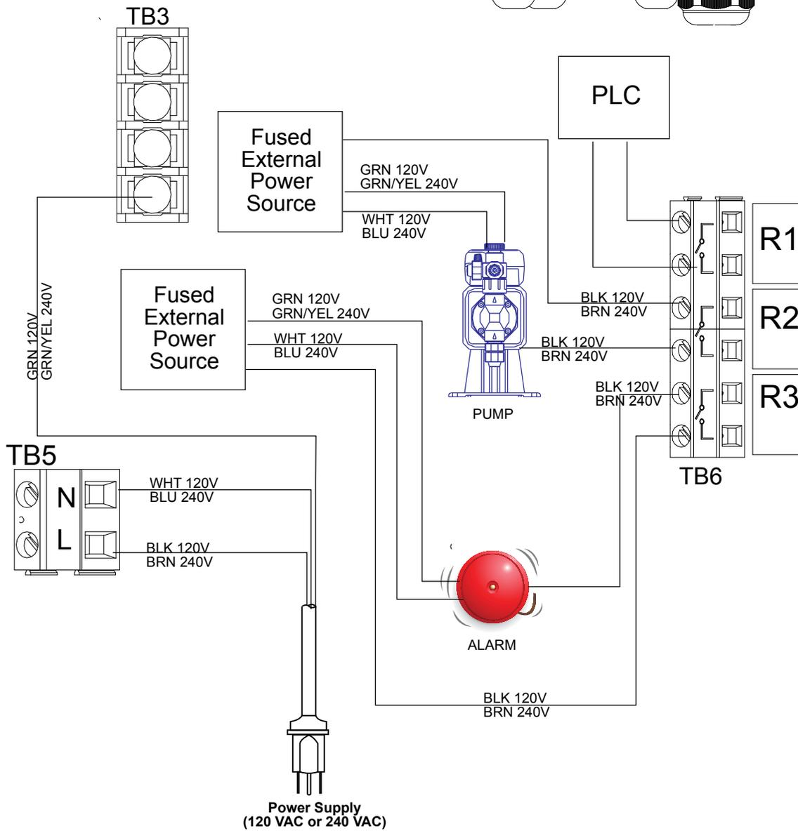
**Figure 14 W110 AC Power & Relay Output Wiring**
