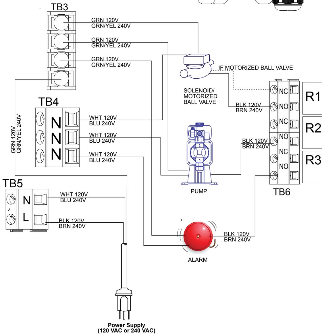
Figure 13 W100 AC Power & Relay Output Wiring
